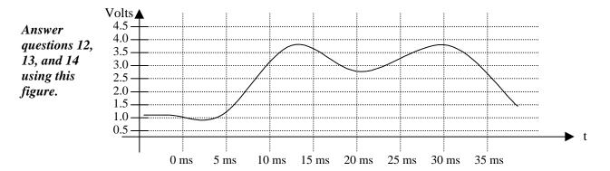
12.) Assuming  $V_{rl}=0.5$  Volts and  $V_{rh}=4.0$  Volts, produce the table of samples output by a three-bit ADC starting at t=0 milliseconds with a sample taken every 5 milliseconds (1 millisecond =  $10^{-3}$  seconds). (5 points)
