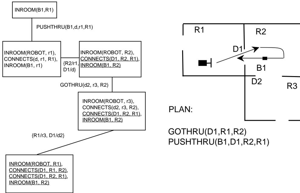
Figure 12.5: A Plan for the Robot Problem
