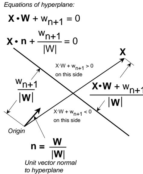
Figure 4.2: TLU Geometry
