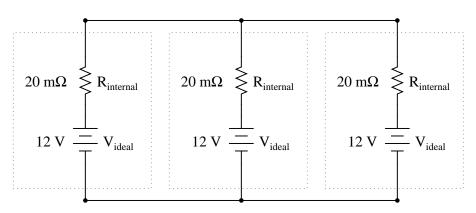
Reduce this network of parallel-connected batteries into either a Thévenin or a Norton equivalent circuit, and then re-calculate the fault current available at the terminals of the three-battery "bank" in the event of a direct short-circuit.
