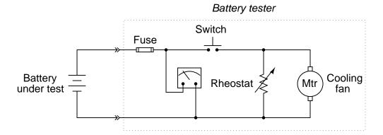
Other clues to the problem include the fact that rheostat setting seems to make no difference in the voltmeter's indication, and also that the cooling fan motor does not come on when the switch is pressed.
