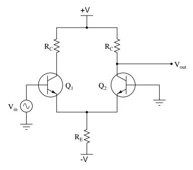
Identify what types of amplifier circuits the two transistors are functioning as (common-collector, common-emitter, common-base) when the differential pair is used like this, and write an equation describing the circuit's voltage gain. Here is another schematic, showing the transistors modeled as controlled current sources, to help you with the equation:
