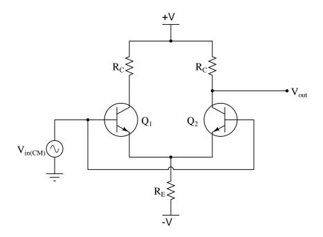
An important performance parameter of any differential amplifier is its common-mode voltage gain. Ideally, a differential-input amplifier should ignore any and all common-mode voltage, but in reality there is always some amplification of common-mode voltage. We need to figure out how much of that there will be in any differential-pair circuit.
