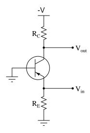
Also, explain how to derive the voltage gain equation for this amplifier:
