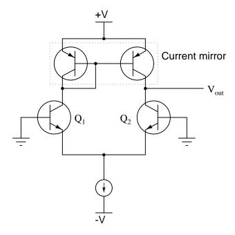
What does the current mirror "look like" to the common-emitter side of the differential amplifier circuit, when we apply the Superposition theorem? What aspect of the differential amplifier's performance is primarily enhanced with the addition of the current mirror to the circuit?
