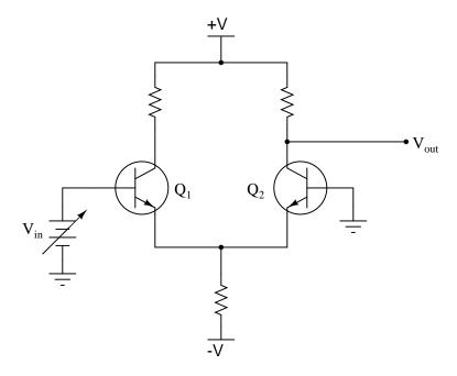
Here, a differential pair circuit is driven by an input voltage at the base of  $Q_2$ , while the output is taken at the collector of  $Q_2$ . Meanwhile, the other input  $(Q_1 \text{ base})$  is connected to ground:
