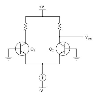
What does the constant-current source "look like" to the rest of the amplifier, in terms of equivalent resistance? What advantage does this give to the amplifier's performance, over the (simpler) resistor design? Finally, how is this constant-current source actually constructed in a typical differential amplifier circuit? file 00936
