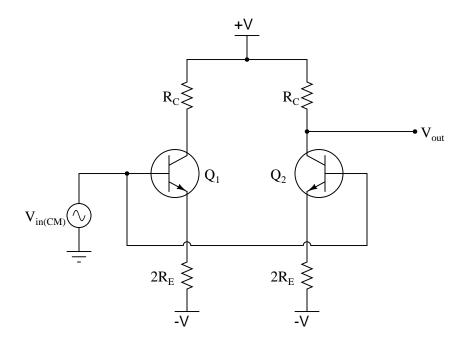
First, explain why this re-drawing is justified, and then write the equation describing the common-mode voltage gain of this circuit, in terms of the component values.
