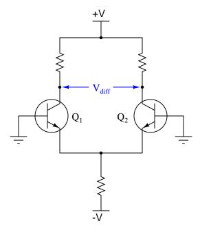
What would happen to this differential voltage  $(V_{diff})$  if transistor Q2 were to increase in temperature, while transistor Q1 remained at the same temperature? Explain your answer.  $\frac{\text{file }00887}{\text{emained }00887}$
