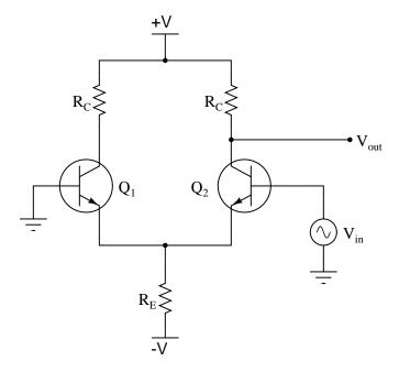
Identify what types of amplifier circuits the two transistors are functioning as (common-collector, common-emitter, common-base) when the differential pair is used like this, and write an equation describing the circuit's voltage gain. Here is another schematic, showing the transistors modeled as controlled current sources, to help you with the equation:
