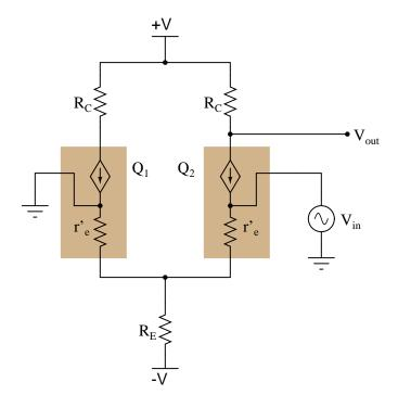
Here, a differential pair circuit is driven by an input voltage at the base of  $Q_1$ , while the output is taken at the collector of  $Q_2$ . Meanwhile, the other input ( $Q_2$  base) is connected to ground:
