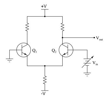
Would you characterize this transistor amplifier as being *inverting* or *noninverting*, with the base terminal of transistor Q1 being considered the input? Explain your answer.
