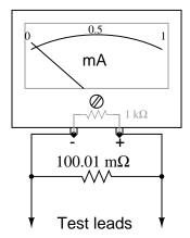
A power dissipation rating of at least 10 watts is necessary for this application.
