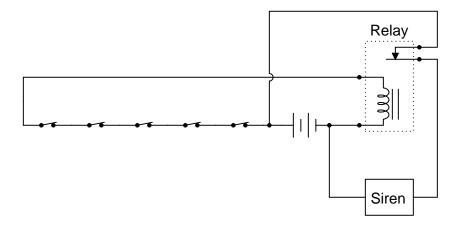
Actuating any of the normally-closed switches results in the alarm sounding. So far, so good. Now, suppose that one of the wires connecting one side of several switches to the rest of the circuit breaks open. What will the result of this failure be?
