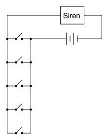
Actuating any of the normally-open switches results in the alarm sounding. So far, so good. Now, suppose that one of the wires connecting one side of several switches to the rest of the circuit breaks open. What will the result of this failure be?
