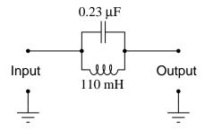
The bandwidth of this 1 kHz notch filter is approximately 29 Hz.
