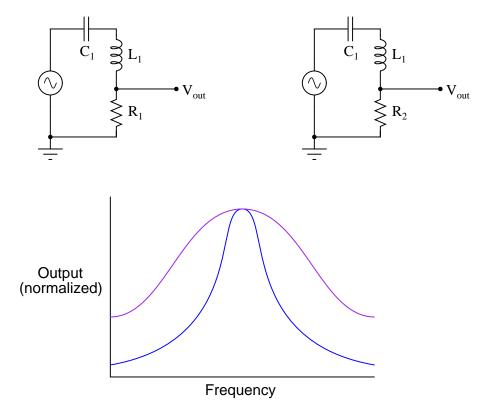
Which one of these plots represents the response of the circuit with the greatest Q, or quality factor?  $\underline{\text{file }01391}$
