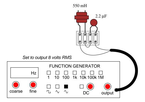
Calculate all voltages and currents in this circuit, at a power supply frequency near resonance:
