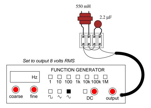
Based on your calculations, what general predictions can you make about parallel-resonant circuits, in terms of their total impedance, their total current, and their individual component currents?  $\frac{\text{file }00609}{\text{file }00609}$
