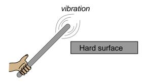
The ability of any physical object to "ring" like this after being struck is dependent upon two complementary properties: *mass* and *elasticity*. An object must possess both mass and a certain amount of "springiness" in order to physically resonate.
