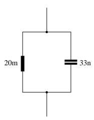
Does a series LC circuit "appear" capacitive or inductive (from the perspective of the AC source powering it) when the source frequency is greater than the circuit's resonant frequency? What about a parallel resonant circuit? In each case, explain why.
