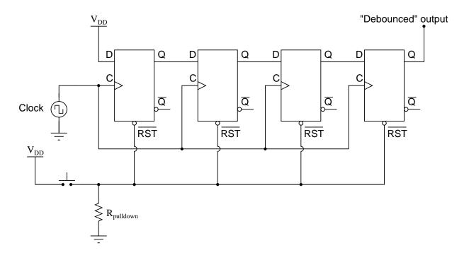
Explain how this circuit works to de-bounce the switch's "dirty" signal, producing a "clean" (de-bounced) signal for a subsequent digital circuit's input.
