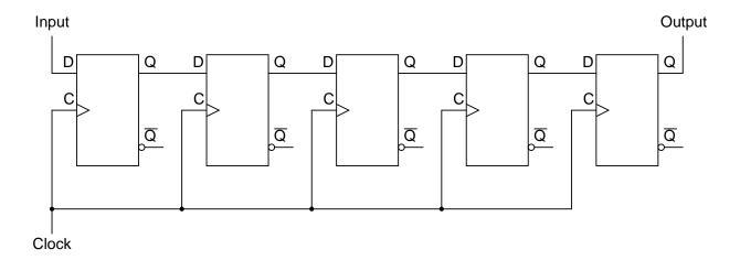
Follow-up question: if we wished to output data from this shift register circuit in parallel form, where would we make the connections?
