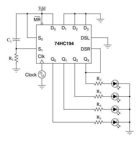
A technician decides to reverse the direction of pattern motion, and alters the circuit as such:
