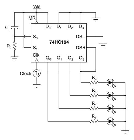
Unfortunately, this does not work as planned. Now, the bottom LED blinks once upon power-up, then all LEDs remain off. What did the technician do that was incorrect? What needs to be done to fix the problem?
