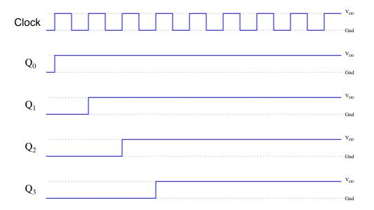
Follow-up question: explain why the "high" state at the D input of the first flip-flop does not ripple through all the flip-flops at the first clock pulse.
