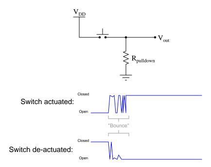
Digital electronic circuits, of course, react to these pulses as though they were very rapid actuations/deactuations of the switch. This may cause problems, especially in applications where a mechanical switch input causes a counter to increment or decrement!
