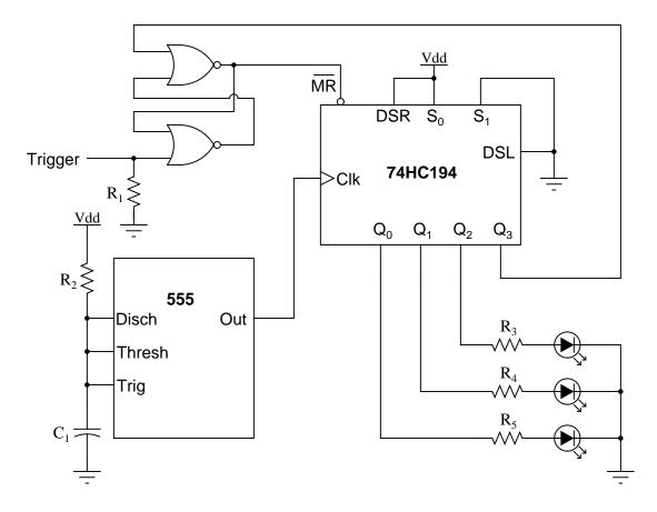
The sequential light pattern is supposed to begin whenever the "Trigger" input momentarily goes high. Unfortunately, something has failed in this circuit which is preventing any of the LEDs to come on. No blinking light sequence ensues, no matter what the state of the "Trigger" input.
