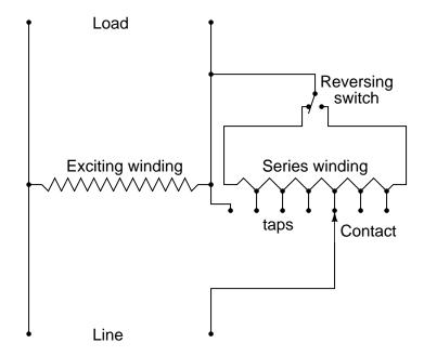
The "Line" side of this autotransformer is the source of power, and the "Load" side connects to those devices consuming electrical power. The "Reversing switch" alters the transformer's function from boost to buck.
