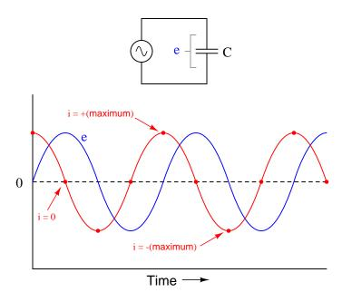
For a capacitor, voltage is lagging and current is leading, by a phase shift of 90°.
