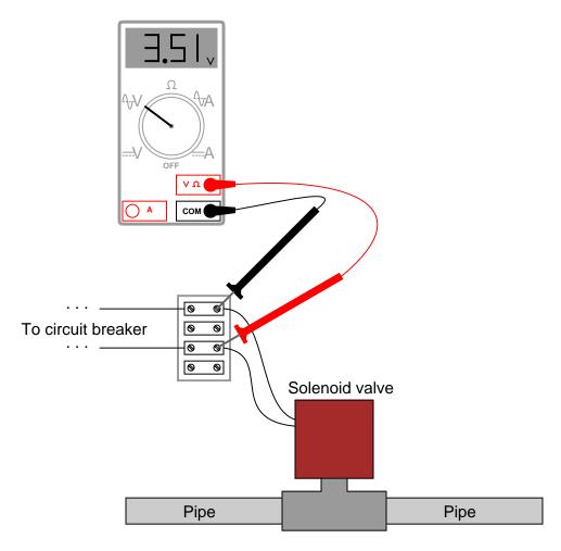
Now, three and a half volts AC is not enough voltage to cause any harm, but its presence confuses and worries the technician. Shouldn't there be 0 volts, with the breaker turned off?
