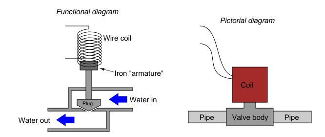
Some solenoid valves are constructed in such a way that the coil assembly may be removed from the valve body, separating these two pieces so that maintenance work may be done on one without interfering with the other. Of course, this means the valve mechanism will no longer be actuated by the magnetic field, but at least one piece may be worked upon without having to remove the other piece from whatever it may be connected to:
