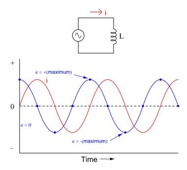
For an inductor, voltage is leading and current is lagging, by a phase shift of 90°.
