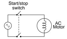
If the voltage of the 60 Hz AC power source is 480 volts RMS, and the motor initially draws 75 amps RMS when the double-pole single-throw switch closes, how much inductance (L) must the motor windings have? Ignore any wire resistance, and assume the motor's only opposition to current in a locked-rotor condition is inductive reactance  $(X_L)$ .
