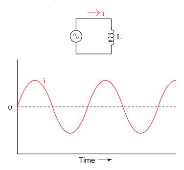
How much phase shift (in degrees) is there between the voltage and current waveforms? Which waveform is leading and which waveform is lagging?
