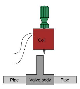
With the steel screwdriver shank taking the place of the iron armature inside the valve body, the coil will not overheat and burn up even if continually powered. Explain the nature of the problem (why the coil tends to burn up when separated from the valve body) and also why a screwdriver put in place of the iron armature works to prevent this from happening.
