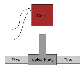
This is commonly done when replacement of the valve mechanism is needed. First, the coil is lifted off the valve mechanism, then the maintenance technician is free to remove the valve body from the pipes and replace it with a new valve body. Lastly, the coil is re-installed on the new valve body and the solenoid is once more ready for service, all without having to electrically disconnect the coil from its power source.
