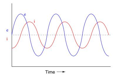
Given that power is the product of voltage and current (p=ie), plot the waveform for power in this circuit. Also, explain how the mnemonic phrase "ELI the ICE man" applies to these waveforms.
