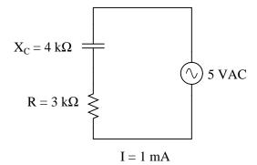
How many ohms of opposition does the series combination of resistor and capacitor offer? What name do we give to this quantity, and how do we symbolize it, being that it is composed of both resistance (R) and reactance (X)?
