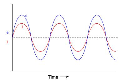
Given that power is the product of voltage and current (p = ie), plot the waveform for power in this circuit.
