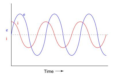
Given that power is the product of voltage and current (p = ie), plot the waveform for power in this circuit. Also, explain how the mnemonic phrase "ELI the ICE man" applies to these waveforms. file 00633
