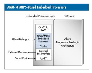
RAM, cache, an external bus interface, and a UART. With these on-chip elements in place, these devices can run software and interface with external components prior to configuration of the programmable logic core. This feature shortens design cycles because software can be written for these devices before developing the programmable logic portion of the design.
