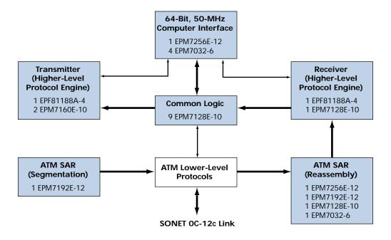
In the ATM OC-12c Protocol Engine, the transmit side processes the data received from the computer, segments it into 53-byte ATM cells, and sends it to the network link. The receiver then reassembles the ATM cells received from the network link, processes the data, and sends it on to the computer.
