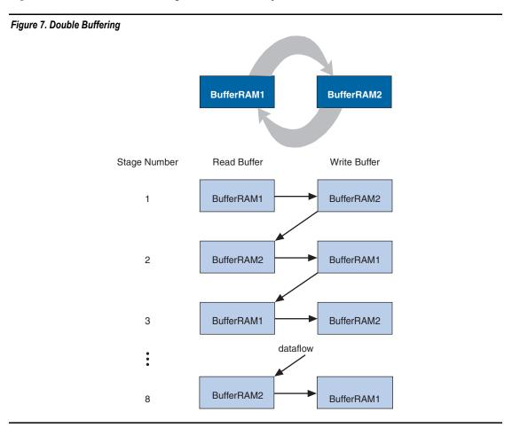
The 256-point FFT in this example decomposes into eight stages. During the first stage the read buffer is **BufferRAM1** and the write buffer is **BufferRAM2**, as shown in Example 1.
