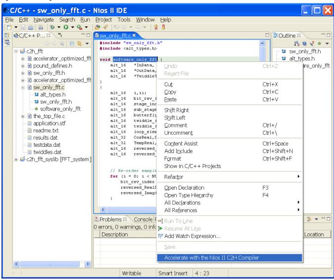
The Nios II compiler displays the following message: ignoring #pragma altera\_accelerate connect\_variable. You can disregard this warning. The C2H Compiler uses the altera\_accelerate pragma to limit the number of master ports, as described in the Restructuring Code to Optimize the Accelerator section. It has no meaning for the Nios II compiler.
