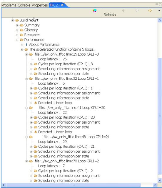
The results in Figure 2 show that most of the values of loop latency and CPLI are high. The next section provides an overview of how the C2H Compiler generates the unoptimized accelerator.
