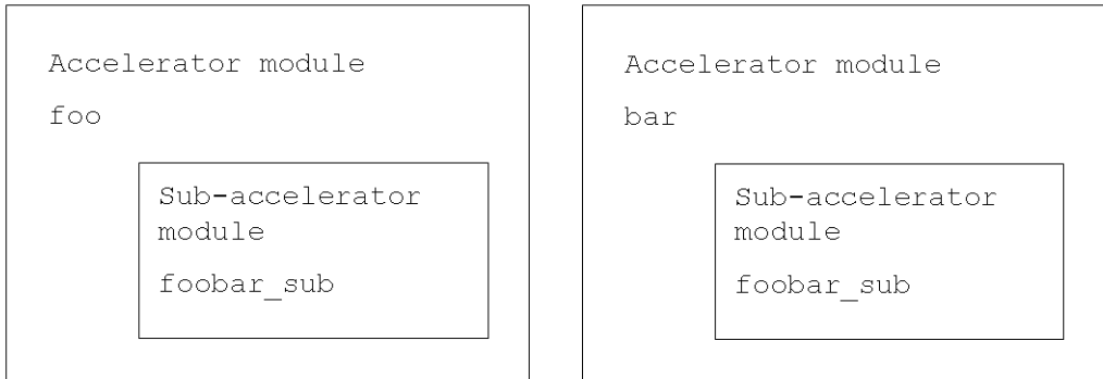
Figure 3-8. Shared Subfunction Logic
