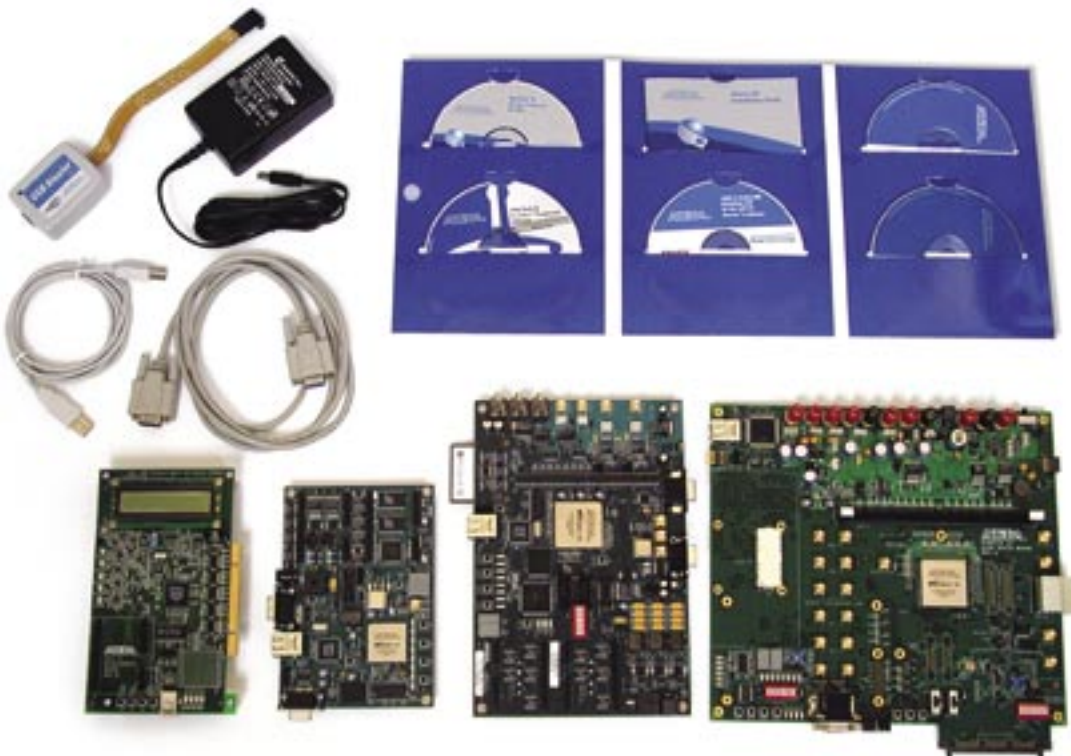
Figure 1. Altera Development Boards (From Left to Right, MAX II, Nios II, Stratix II DSP, & Stratix II High-Speed Development Boards)
