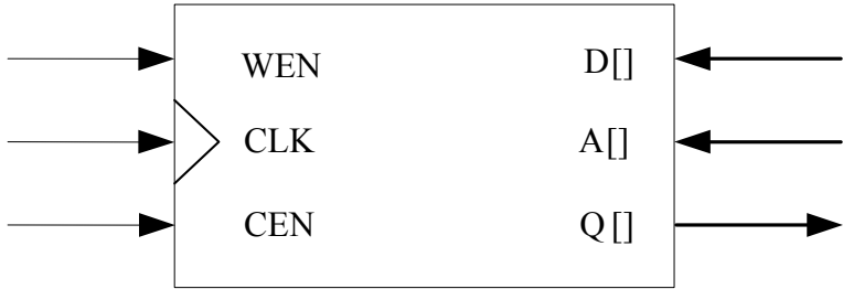
Figure 2.4.5 Single-port Memory Mode
