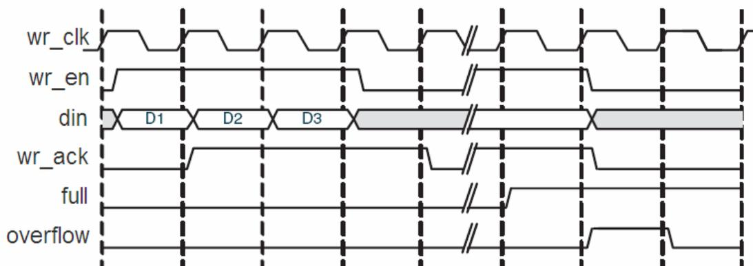
**Figure 6 Write acknowledge signal for Asynchronous FIFO**
