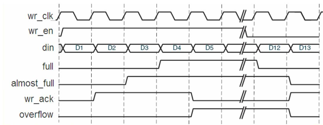
Figure 3 Write Operation for a Asynchronous FIFO
