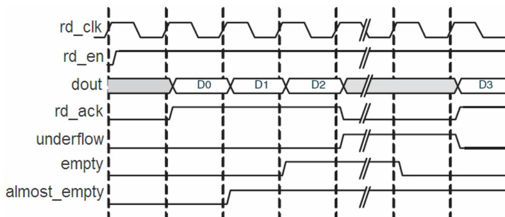
Figure 4 Read Operation for a Asynchronous FIFO
