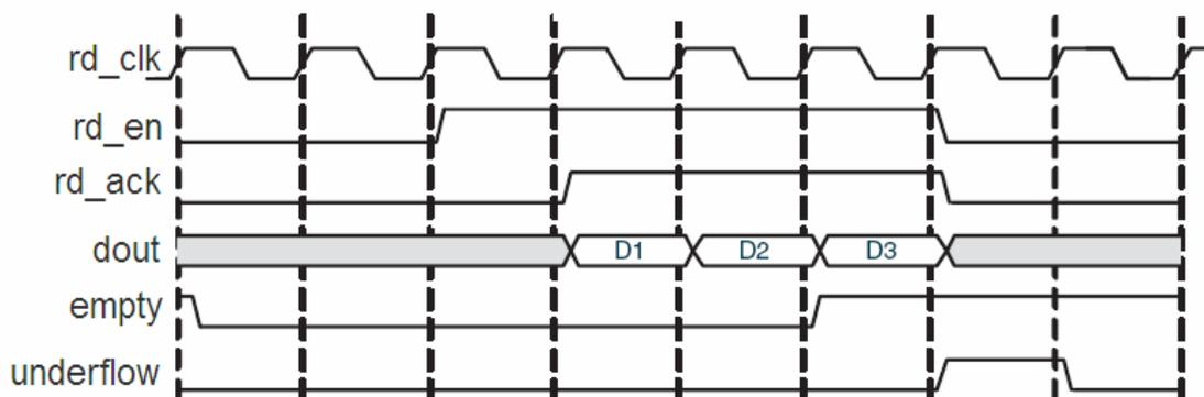
Figure 8 Underflow Signal for Synchronous FIFO
