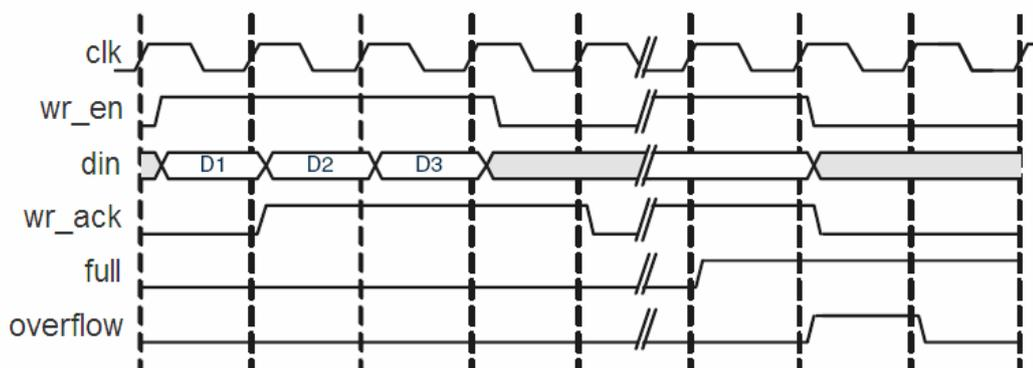
Figure 10 Write Acknowledge Signal for Synchronous FIFO
