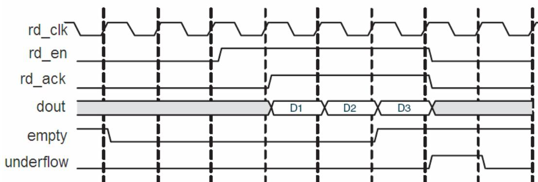
**Figure 7 Read Acknowledge Signal for Asynchronous FIFO**
