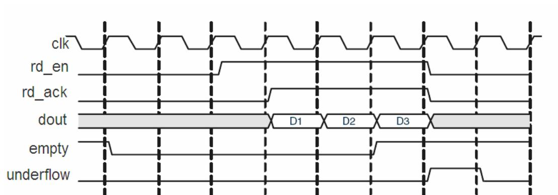
**Figure 11 Read Acknowledge Signal for Synchronous FIFO**
