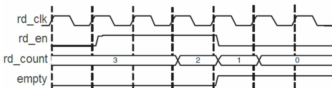
**Figure 22 Read Data Count for Asynchronous FIFO**
