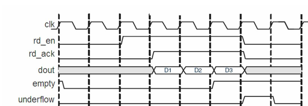
**Figure 12 Underflow Signal for Synchronous FIFO**
