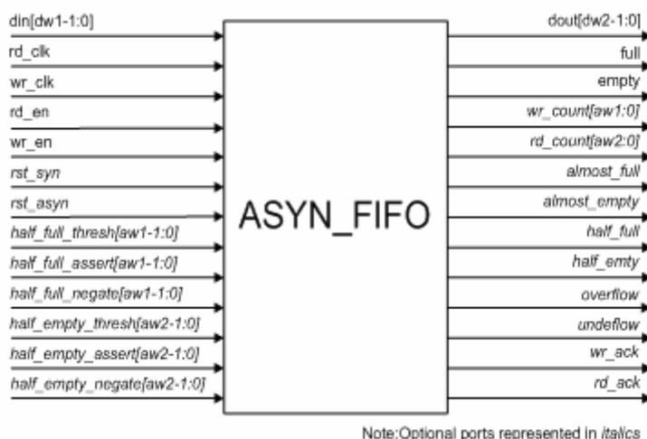
**Figure 1 Asynchronous FIFO Interfaces**
