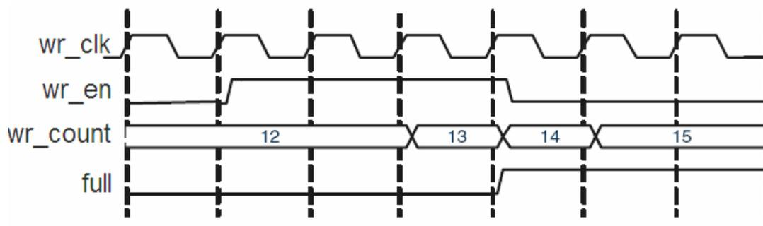
Figure 23 Write Data Count for Asynchronous FIFO
