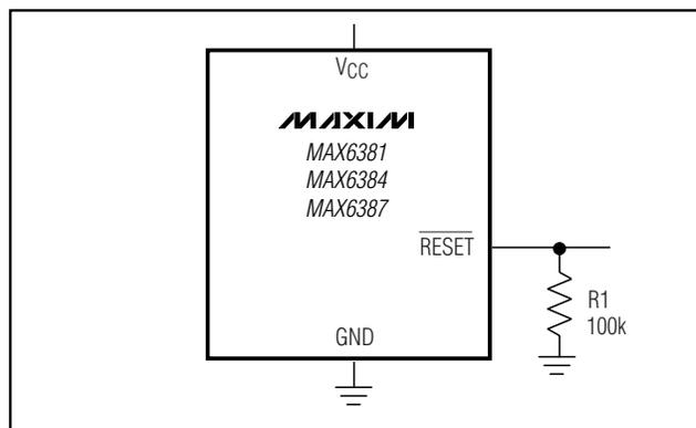
Figure 2. RESET Valid to  $V_{CC} = \text{Ground}$  Circuit
