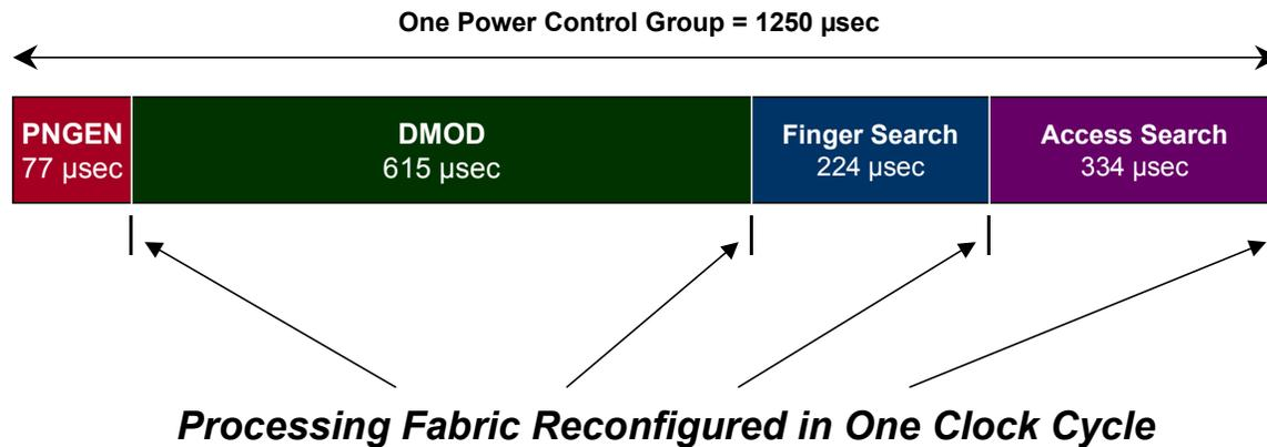
**Figure 3 – Chip-rate Processing Using eConfigurable Technology**
