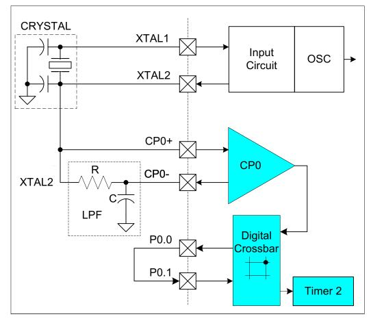
Figure 1. Connection Diagram
