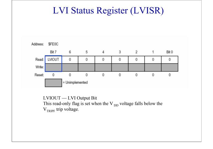
The LVI Module uses the LVI status register (LVISR) to indicate when the V<sub>DD</sub> voltage falls below the V<sub>TRIPF</sub> level. The LVI output bit, LVIOUT, is a read-only status flag that the LVI Module sets when V<sub>DD</sub> is less than V<sub>TRIPF</sub>. The LVI Module clears the bit when V<sub>DD</sub> rises above V<sub>TRIPR</sub>. A reset clears the LVIOUT bit.
