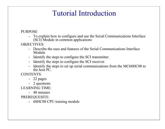
Welcome to this tutorial on the 68HC08 Serial Communications Interface (SCI) Module. This tutorial describes the features and configuration of the SCI Module. Please note that on subsequent pages, you will find reference buttons in the upper right of the content frame that access additional content.
