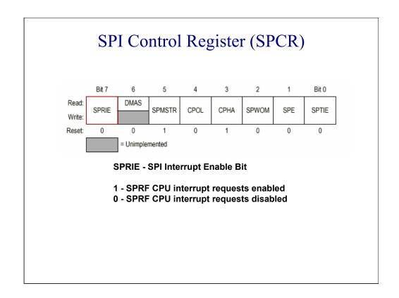
The clock phase bit, CPHA, is a read/write bit that controls the timing relationship between the serial clock and SPI data. To transmit data between two SPI modules, the SPI modules must have identical CPHA values. We will examine phase and polarity later in the tutorial.
