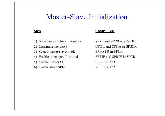
Next, let's review the steps to configure the SPI for data transmission using SPSCR and the SPCR.
