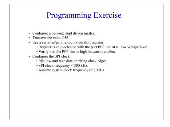
Let's complete this tutorial with an off-line programming exercise. Let's write a program to configure the master SPI for data transmission. In this exercise, we'll perform a polled SPI transfer of one byte to a serial-in/parallel-out 8-bit shift register. We could use this program to provide additional latched I/O ports through the shift register.
