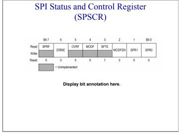
The SPI Status and Control Register, SPSCR, contains status flags and additional control bits.
