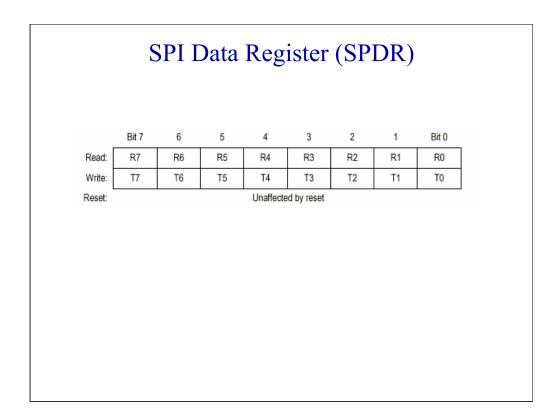
The SPI data register is actually two registers that you access with one address. The two registers are the receive data register and the transmit data register. These are separate registers that contain different values. You access the individual registers using the read/write actions. Reading the SPI data register reads data from the receive data register. Writing to the SPI data register writes data into the transmit data register.
