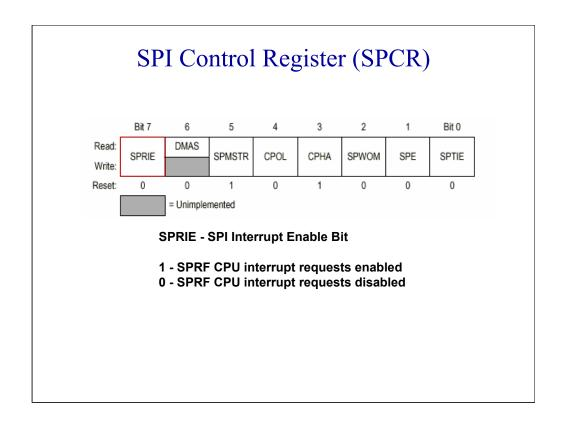
The figure shows the the SPI control register, SPCR. Let's review each control bit in detail.
