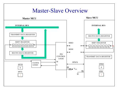
The SPI is built around a double buffered 8-bit shift register with both ends of the shift register brought out to MCU pins. One end of the shift register is connected to the master-in slave-out pin, MISO. This pin acts as an input for the master SPI Module and as an output for the slave SPI Module. The other end of the shift register is connected to MOSI pin.
