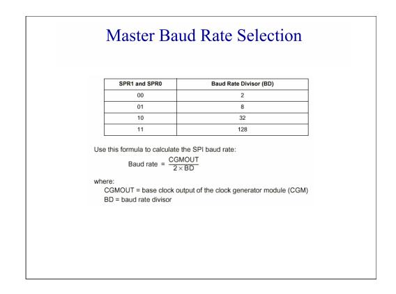
Let's take a closer look at how the baud rate is calculated. The table shows the bit codes for selecting one of four baud rate divisors using the SPI baud rate select bits (SPR1 and SPR0). The baud rate is calculated by dividing the bus frequency by two times the baud rate divisor.
