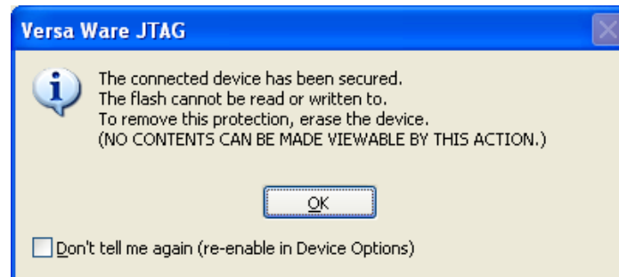
Figure 13: A Secured Device
