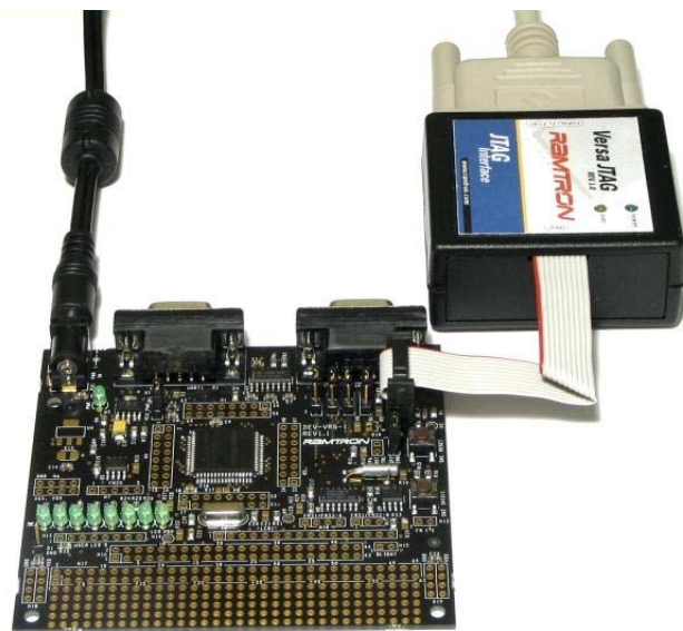
Figure 11: Connecting the Versa-JTAG programming interface and the development board supply
