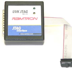
Figure 10: Versa-JTAG interface for programming and debugging the VRS51L3074
