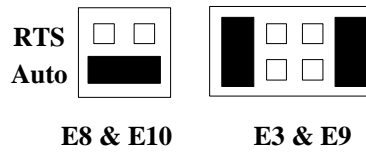
Figure 8 - RS-485 'Auto' Enabled, with 'Echo'
