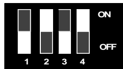
Figure 4 - Dip switch SW-1
