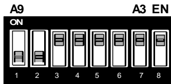
Figure 2 - DIP-Switch SW2 Illustration
