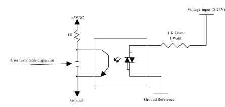
The opto-isolator has two 'back-to-back' diodes internally. This allows AC or DC signals to be sensed, regardless of polarity. When the applied voltage is high enough to cause the LED in the opto-isolator to turn-on, the output of the opto-isolator goes low (0 volts) and the signal is read as a low logic level (binary 0) by the PC. When the input signal is too low to turn on the opto-isolator, the output goes high and the port bit is read by the PC as a high logic level (binary 1).
