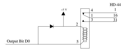
The above is a schematic representation of the Output Bit D0. The NC contact would be Pin 1 on the HD44, N0 would be Pin 31 and the Common would be Pin 16.
