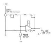
**Figure 4**. Example circuit for an AD590 sensor that uses an OP177 operational amplifier (op amp) to provide higher voltages to an ADC or other measurement circuit. (Courtesy of Analog Devices.)
