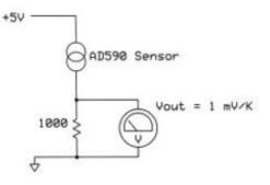
**Figure 1**. The current from this AD590 sensor passes through a precision 1000-ohm resistor. The resulting voltage represents temperature at a rate of 1 mV/K. So at 20°C (293K), you would measure 293 mV at the circuit output.
