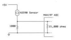
**Figure 2**. The connection of an AD590 sensor and MAC197 ADC creates a circuit with two resistances in parallel.
