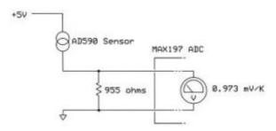
Figure 3. The equivalent circuit for the AD590 sensor and the MAX197 ADC.
