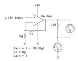
**Figure 5**. Test circuit for an op-amp output impedance, or resistance. In this circuit the non-inverting op-amp configuration amplifies the 1.10-volt signal by two.
