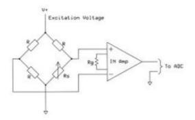
**Figure 6**. This bridge circuit indicates a resistance change in the sensor element (Rs) as a voltage difference between the two output signals applied to the in amp. The amplifier removes any common-mode voltage from the excitation source and puts out only the voltage difference between the two inputs. Resistor Rg determines the in-amp's gain.
