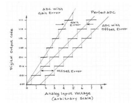
**Figure 6**. Plots of ADC behavior that show a gain error and an offset error in the digital outputs. These plots exaggerate the errors for the sake of clarity.
