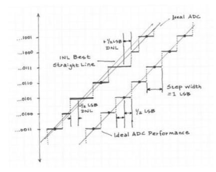
**Figure 5**. Plots for an ideal ADC (right) and for an ADC that shows differential and integral nonlinearity errors.
