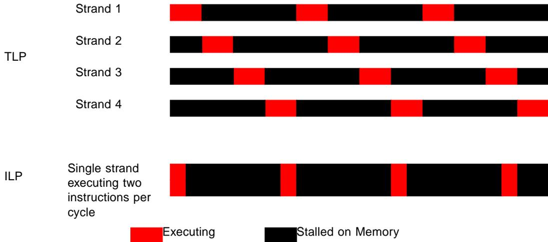
The memory stall time of one strand can often be overlapped with execution of other strands on the same processor, and multiple processors run their strands in parallel. In the ideal case, shown in FIGURE 1-1, memory latency can be completely overlapped with execution of other strands. In contrast, instruction-level parallelism simply shortens the time to execute instructions and does not help much in overlapping execution with memory latency.<sup>1</sup>
