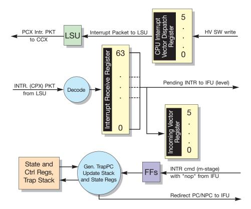
FIGURE 2-31 Flow of Hardware and Vector Interrupts
