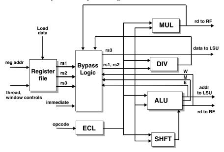
FIGURE 2-15 Execution Unit Diagram
