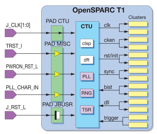
FIGURE 10-1 Clock and Reset Functional Block Diagram
