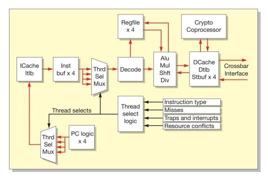
FIGURE 1-2 SPARC Core Pipeline
