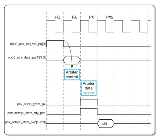
FIGURE 3-4 PCX Packet Transfer Timing – One Packet Request
