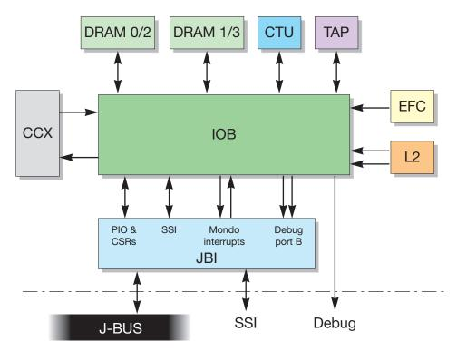
FIGURE 5-1 IOB Interfaces
