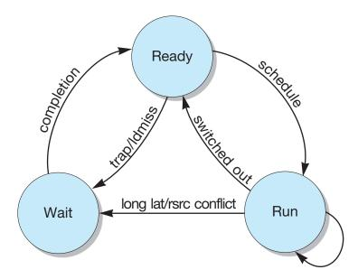
FIGURE 2-10 Thread State Transition of an Active Thread
