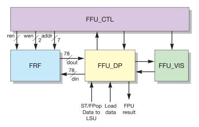
FIGURE 2-19 Top-Level FFU Block Diagram
