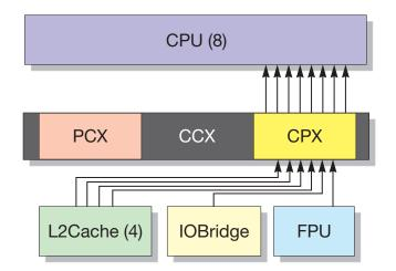
FIGURE 3-3 Cache-Processor Crossbar (CPX) Interface
