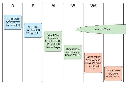
FIGURE 2-29 Trap Flow Sequence
