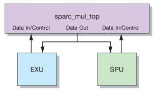
FIGURE 2-20 Multiplexor (MUL) Block Diagram
