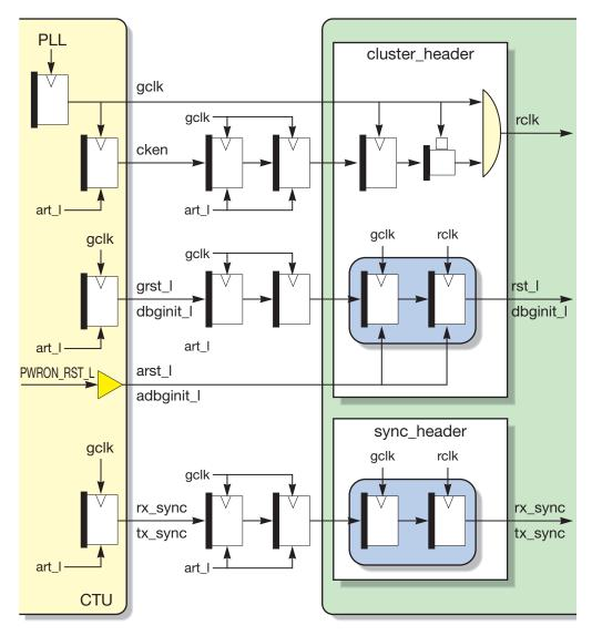
FIGURE 10-5 Clock Signal Distribution
