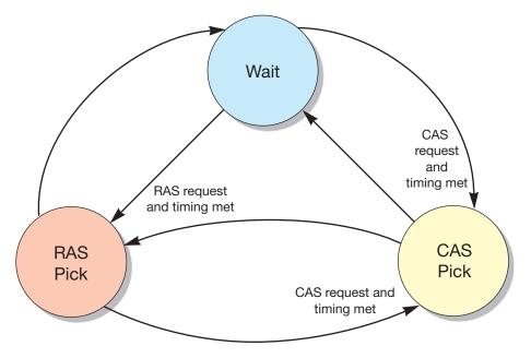
FIGURE 8-3 DIMM Scheduler State Diagram
