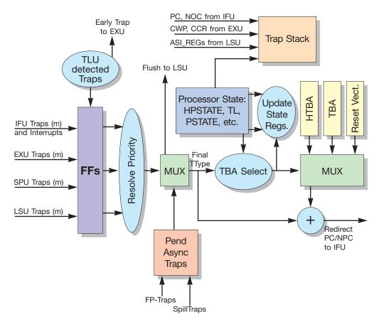
FIGURE 2-30 illustrates the trap flow with respect to the hardware blocks.
