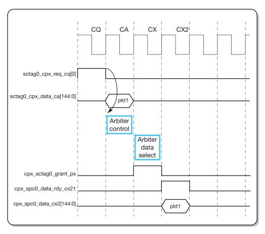
FIGURE 3-6 CPX Packet Transfer Timing Diagram – One Packet Request
