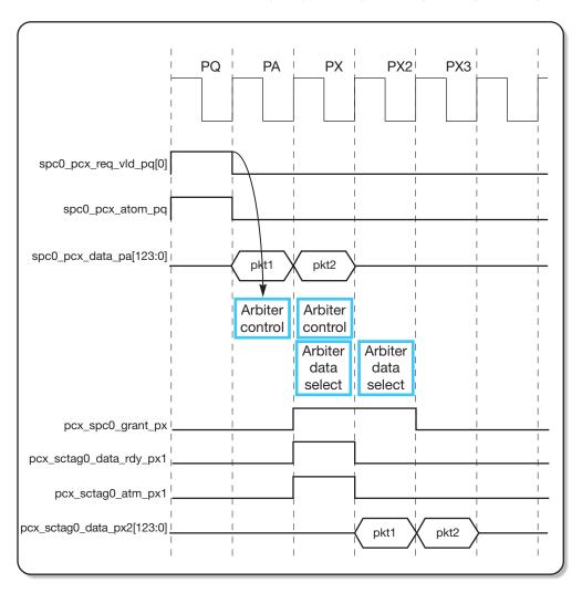
FIGURE 3-5 shows timing diagram for processing a two-packet request.
