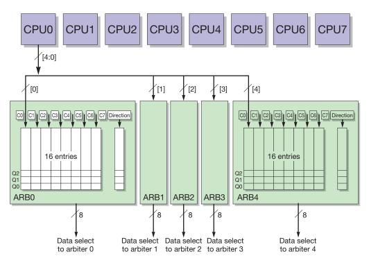
FIGURE 3-12 Control Flow in PCX Arbiter
