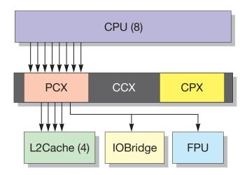
FIGURE 3-2 Processor Cache-Crossbar (PCX) Interface
