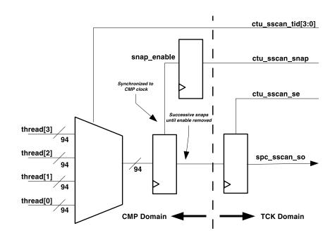
FIGURE 2-37 SPARC Shadow Scan Chain
