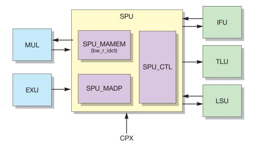
FIGURE 2-22 Data Flow of Modular Arithmetic Operations
