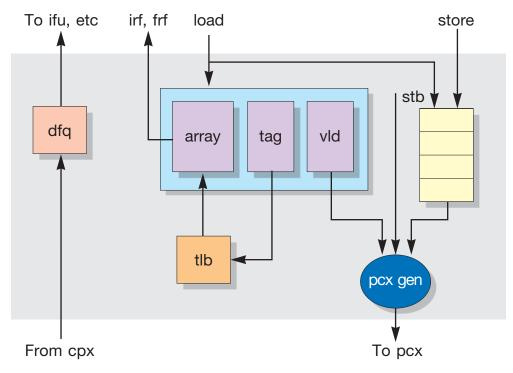
FIGURE 2-14 LSU Data Flow Concept
