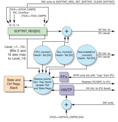
FIGURE 2-33 illustrates the flow of software and timer interrupts.
