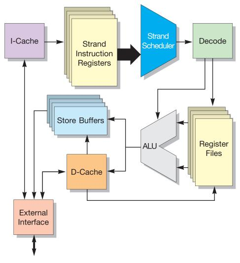
FIGURE 2-1 SPARC Core Block Diagram
