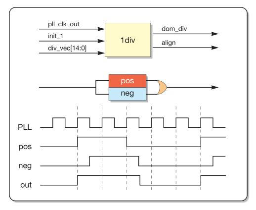
FIGURE 10-3 Clock Divider Block Diagram
