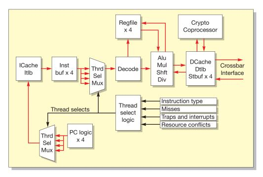
FIGURE 2-4 SPARC Core Pipeline and Support Structures
