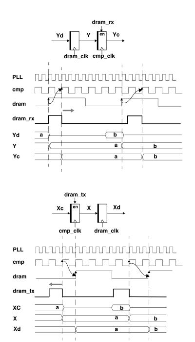
FIGURE 10-4 Sync Pulses Waveforms
