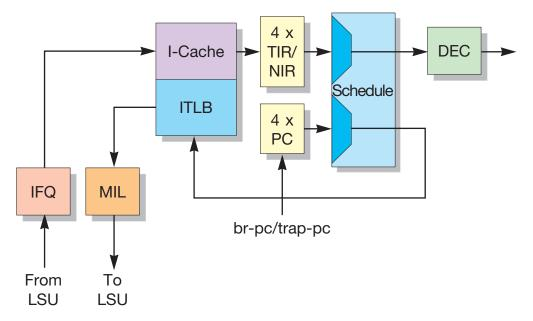
FIGURE 2-5 Frontend of the SPARC Core Pipeline
