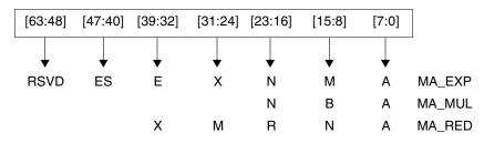
FIGURE 2-21 Layout of MA\_ADDR Register Bit Fields
