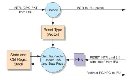
FIGURE 2-32 illustrates the flow of reset, idle, or resume interrupts.
