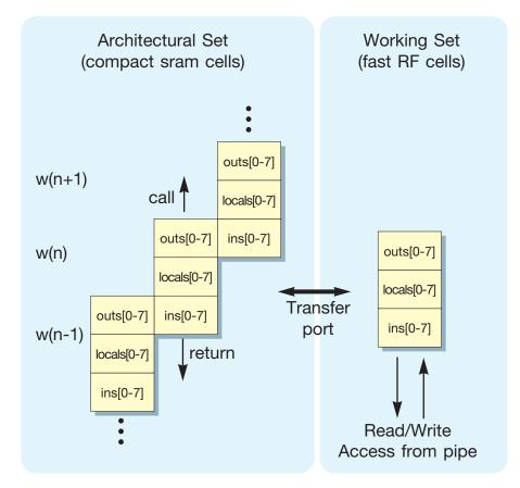
FIGURE 2-8 IARF and IWRF File Structure
