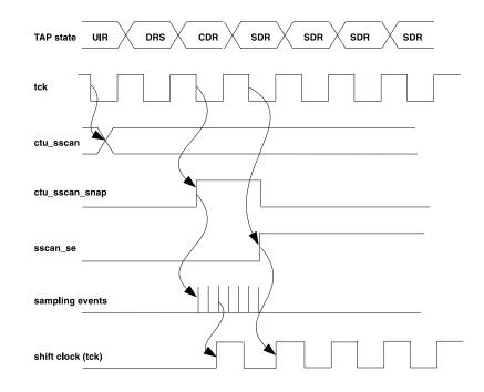
FIGURE 2-38 Shadow Scan Snap Timing Diagram
