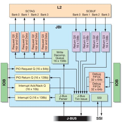
FIGURE 6-1 displays the JBI block diagram.
