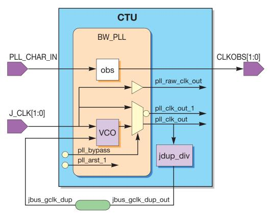
FIGURE 10-2 PLL Functional Block Diagram
