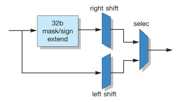
FIGURE 2-16 Shifter Block Diagram
