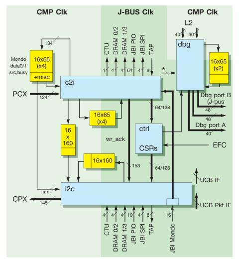
FIGURE 5-3 IOB Internal Block Diagram
