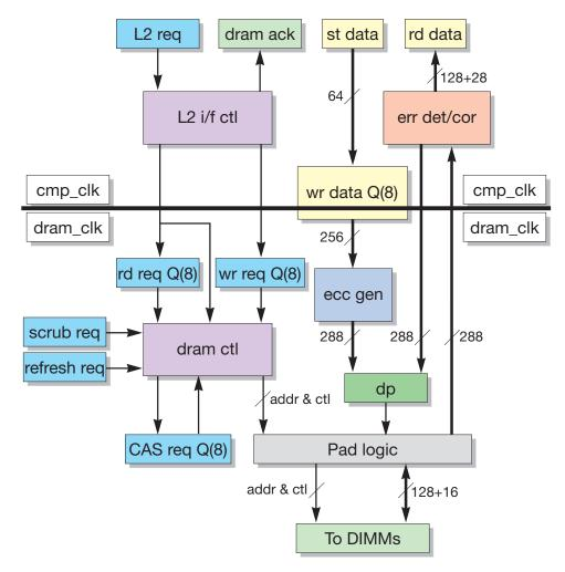
FIGURE 8-1 DDR-II DRAM Controller Functional Block Diagram
