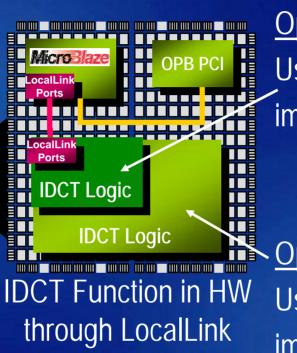
Option 1: Use small (200 LUTs) implementation of IDCT in HW – only 107 clock cycles - 10x faster Option 2: Use fast (1,600 LUTs) implementation of IDCT in HW - only 52 clock cycles – 22x faster
