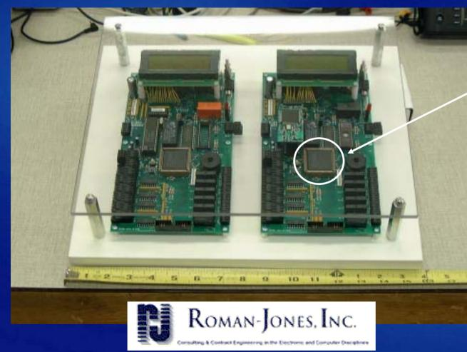
Spartan-II FPGA (XC2S30) featuring PicoBlaze to emulate 8051 operation
