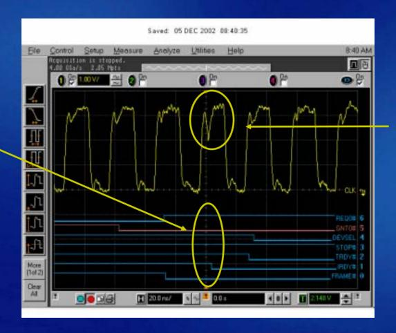
Analog channels see isolated clock coupling
