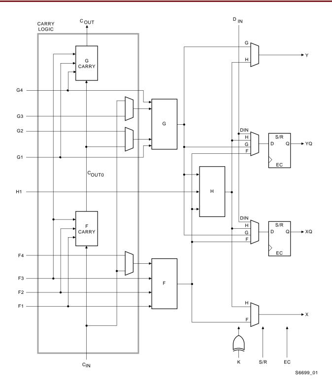
Figure 15: Fast Carry Logic in Spartan CLB
