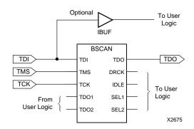
Figure 21: Boundary Scan Schematic Example
