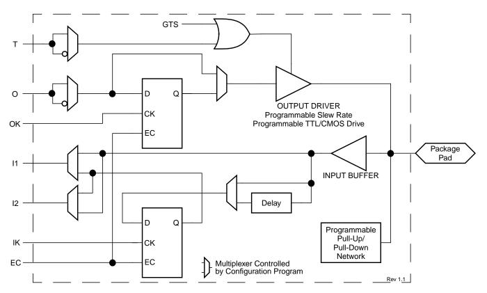
Figure 5: Simplified Spartan IOB Block Diagram
