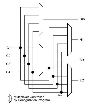
Figure 4: CLB Control Signal Interface
