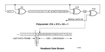
Figure 25: Circuit for Generating CRC-16
