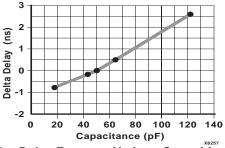
Figure 28: Delay Factor at Various Capacitive Loads
