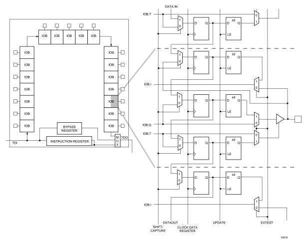
Figure 19: Spartan Series Boundary Scan Logic
