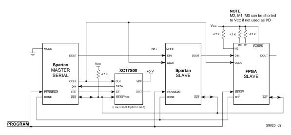
Figure 23: Master/Slave Serial Mode Circuit Diagram
