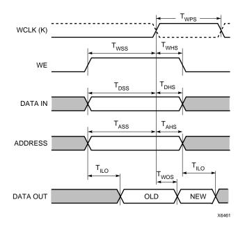
Figure 12: Data Write and Access Timing for RAM
