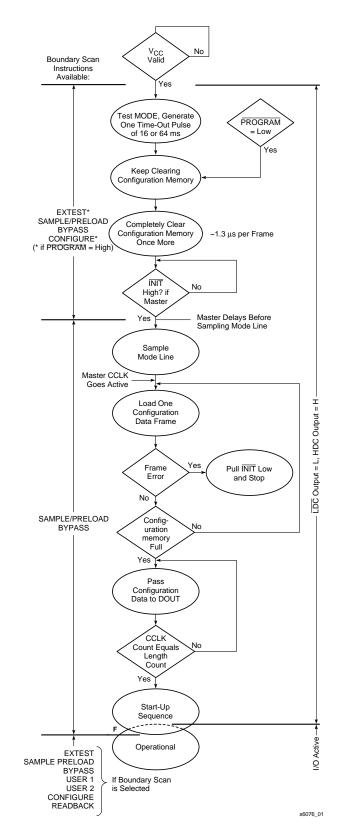
Figure 26: Power-up Configuration Sequence
