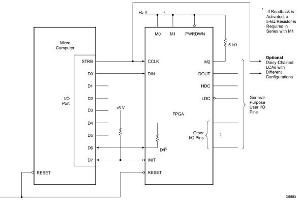
Figure 29: Slave Serial Mode Circuit Diagram
