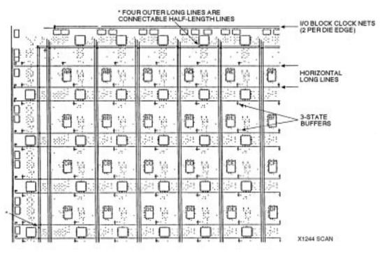
**Figure 15: Programmable Interconnection of Longlines.** This is provided at the edges of the routing area. Threestate buffers allow the use of horizontal Longlines to form on-chip wired AND and multiplexed buses. The left two nonclock vertical Longlines per column (except XC3020A) and the outer perimeter Longlines may be programmed as connectable half-length lines.
