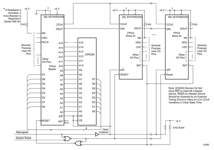
Figure 25: Master Parallel Mode Circuit Diagram
