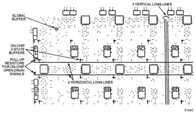
**Figure 14:** Horizontal and Vertical Longlines. These Longlines provide high fan-out, low-skew signal distribution in each row and column. The global buffer in the upper left die corner drives a common line throughout the FPGA.
