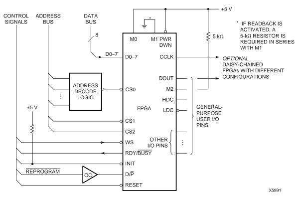
Figure 27: Peripheral Mode Circuit Diagram
