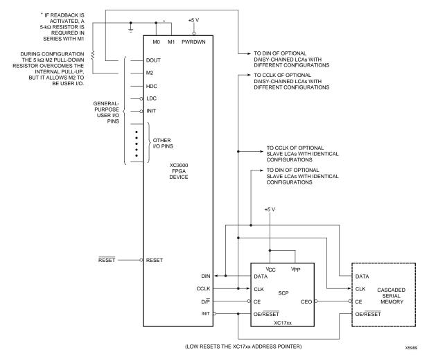
Figure 23: Master Serial Mode Circuit Diagram
