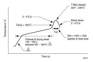
Figure 4: Typical conditions for IR reflow soldering
