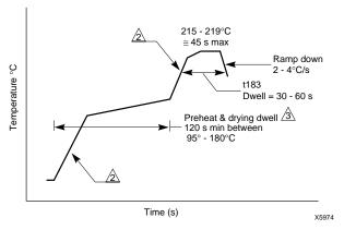
**Figure 5:** Typical conditions for vapor phase reflow soldering
