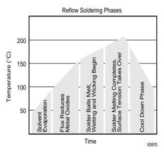
Figure 2: Soldering Sequence
