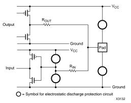
Figure 3: Input/Output Protection Circuity
