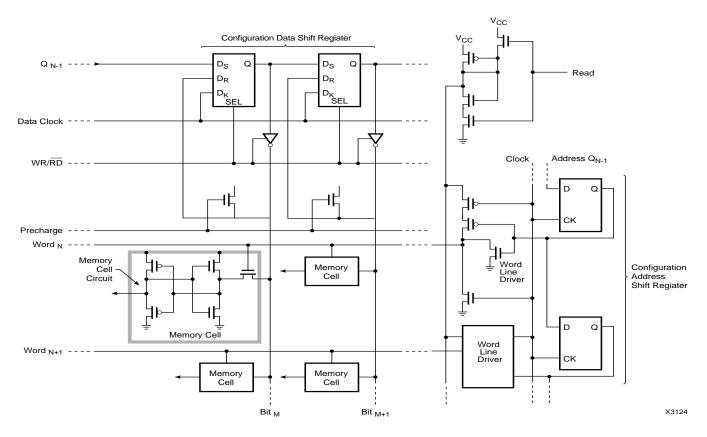
Figure 2: Configuration Memory Cell
