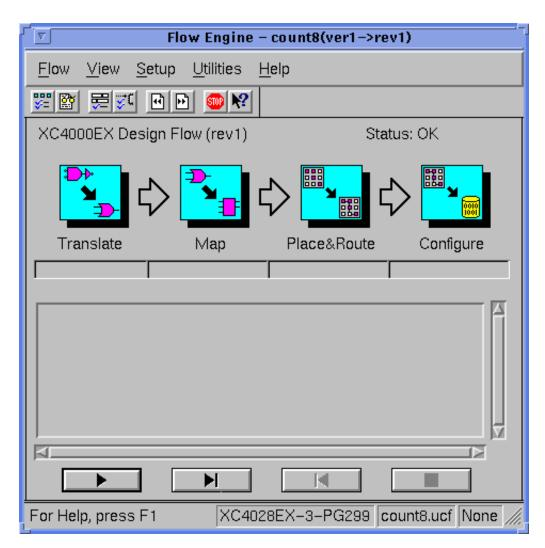
Figure 3-4 Flow Engine With "count8.ucf" Selected
