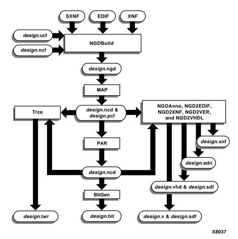
Figure 4-2 Detailed Design Flow
