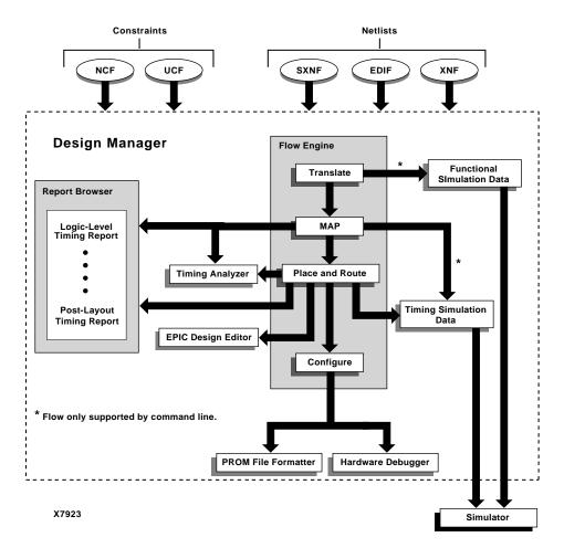
Figure 4-1 M1 Software Design Flow
