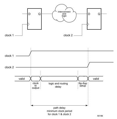
Figure 2-5 Clock-to-Setup Path (Different Clocks)
