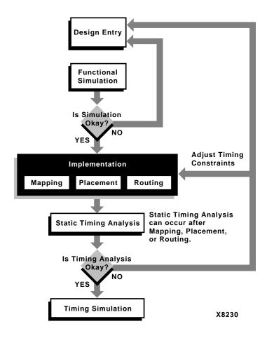
Figure 1-1 Timing Analyzer in the Design Flow
