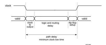
Figure 2-4 Clock-to-Setup Path (Falling to Rising Edge)
