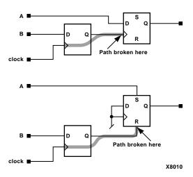
Figure 2-9 Clock-to-Pad Path Broken Through Set/Reset Inputs
