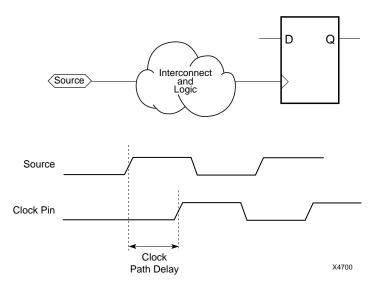
Figure 2-10 Paths Ending at Clock Pin of Flip-Flops
