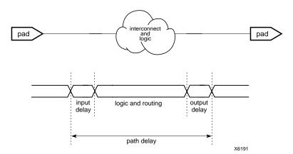
Figure 2-12 Pad-to-Pad Delay
