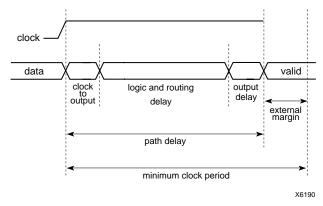
Figure 2-7 Clock-to-Pad Path
