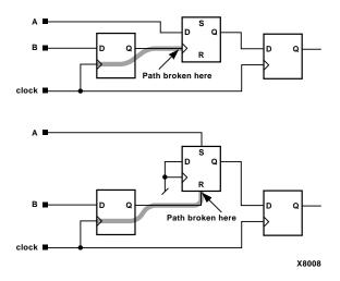
Figure 2-6 Not Propagating Through Asynchronous Set/Reset
