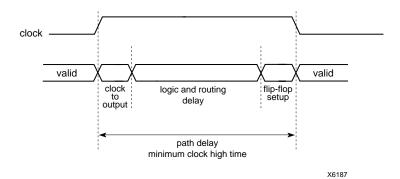
Figure 2-3 Clock-to-Setup Path (Rising to Falling Edge)
