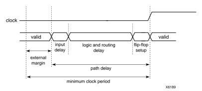
Figure 2-14 Pad-to-Setup Path
