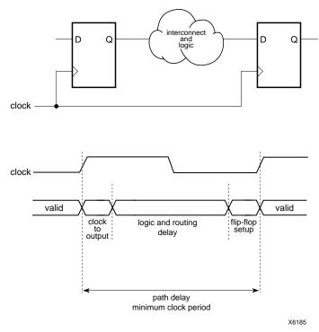
Figure 2-2 Clock-to-Setup Path (Same Clock) with Timing Diagram
