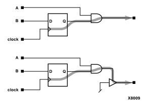
Figure 2-8 Through Tristate Controlled Pads
