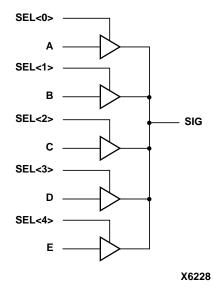
Figure 4-11 5-to-1 MUX Implemented with BUFTs
