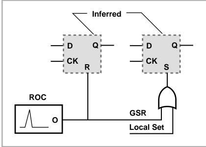
Figure 5-3 ROC Simulation and Implementation
