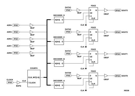
Figure 4-7 Schematic Block Representation of I/O Decoder
