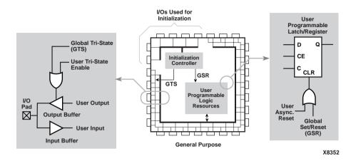
Figure 5-2 Built-in FPGA Initialization Circuitry
