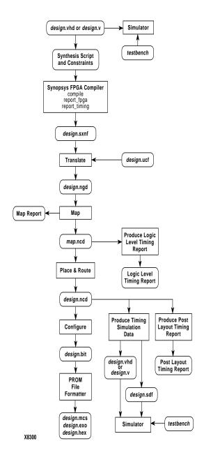
Figure 3-2 Design Flow Using the Design Manager
