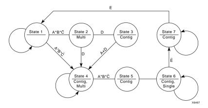
Figure A-1 A TYPICAL STATE MACHINE BUBBLE
