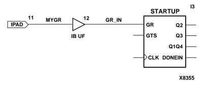
Figure 5-9 Verilog User-Controlled Inverted GR
