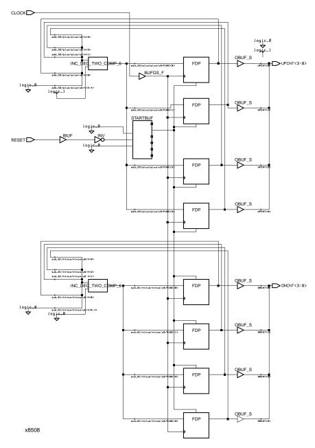
Figure 4-5 Use\_GSR Implemented with Gates
