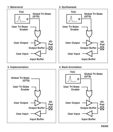
Figure 5-5 TOC Simulation and Implementation
