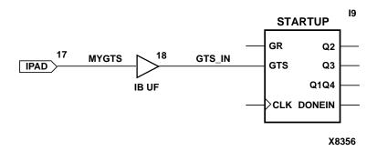
Figure 5-10 Verilog User-Controlled Inverted GTS
