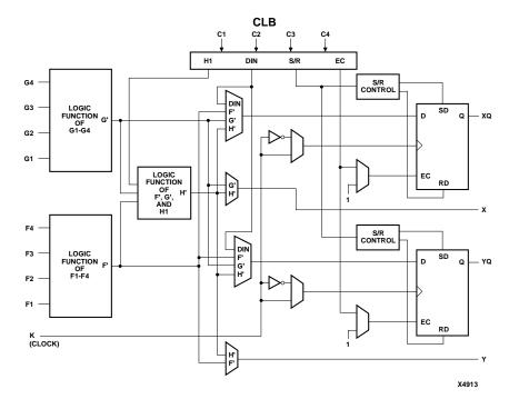
Figure 2-7 XC4000 Configurable Logic Block
