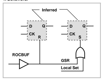
Figure 5-4 ROCBUF Simulation and Implementation
