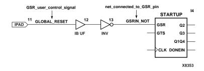
Figure 5-7 Verilog User-Controlled Inverted GSR
