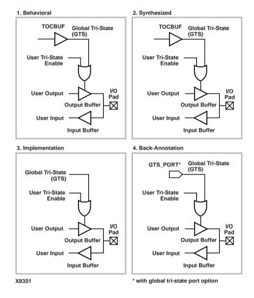
Figure 5-6 TOCBUF Simulation and Implementation
