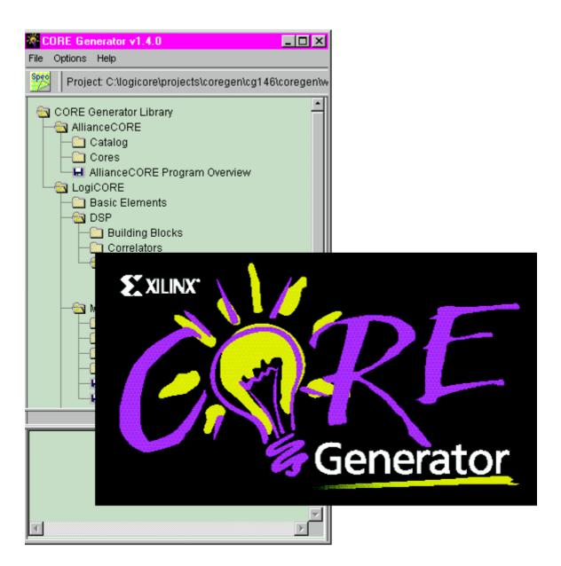
The Xilinx CORE Generator, presents the designer with a catalog of ready-made functions ranging in complexity from simple arithmetic operations such as adders, accumulators, and multipliers, to system-level building blocks, including filters, transforms, and memories. Selecting the desired function, or module, is simplified by the tree-like presentation of the catalog, where modules of a similar type are grouped together in folders that expand or contract on demand.
