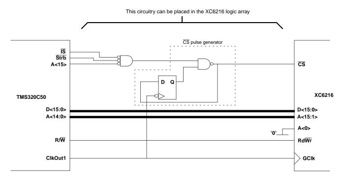
Figure 3. Basic Example Circuit
