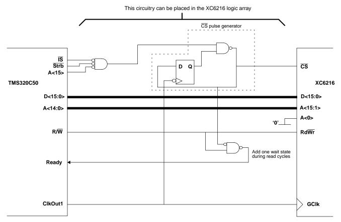
Figure 7. Example Circuit With External Wait State Generator
