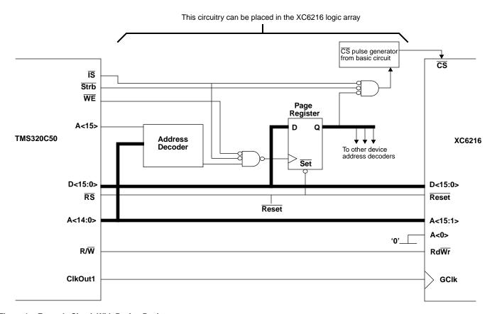
Figure 4. Example Circuit With Paging Register
