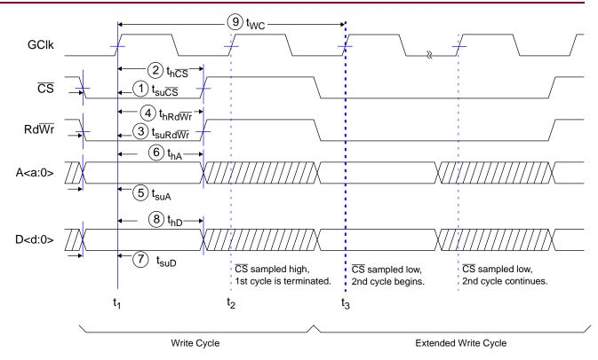
Figure 1. XC6200 Write Cycles
