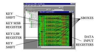
Figure 5: XACT6000 layout of Encryption Design
