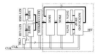
Figure 2: Structure of DES Encryption Design
