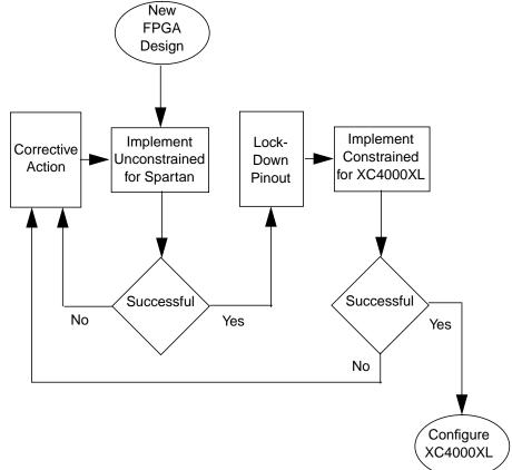
Figure 2: Design Implementation Flow for XC4000XL Prototype
