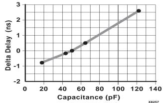
Figure 1: Delay Factor at Various Capacitive Loads
