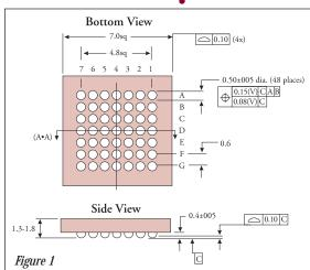
CSPs can benefit from CPLD speed and cost improvements (die shrinks) without ever having to change package footprint, because die shrinks can be accommodated without having to change package dimensions.
